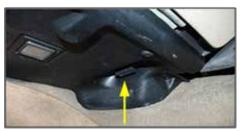
**For the Classic:** In this order, firstly plug the 15 pin D connector of the diagnostic lead into the EAS Kicker Lite. Then locate the Black EAS diagnostic connector in the pocket under the Driver's seat and disconnect the looped plug from this. Insert the Red plug of the diagnostic cable into the Black socket. Plug the power lead into the power source of the vehicle (cigar lighter) and then plug the other power lead into the EAS Kicker Lite's DC jack socket.
