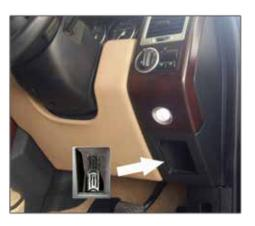
As soon as the EAS Kicker Lite is plugged in correctly, the LED will illuminate with a solid BLUE light. This means the unit is working and is speaking to the EAS system. When it has done this, you will observe a sequence of Green or Red lights from the LED which are interpreted as follows:
