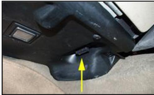
As soon as the BeCM Sync-Mate is plugged in correctly, the LED will illuminate with a solid **BLUE** light. This means the unit is working and is attempting to communicate with the BeCM and the relevant Engine Management System. When it has done this, you will see a sequence of solid or flashing **Green** (EDC or MOTRONIC only), alternating **Green/Blue** (Gems Only) or Flashing **Red** lights from the LED.
